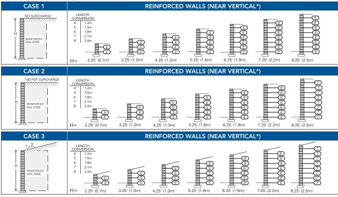
\*FOR CONSTRUCTION OF NEAR VERTICAL BATTER (CENTER PIN HOLE), CONSTRUCT WITH POSITIVE BATTER BY TILTING UNITS BACK TOWARDS FILL ON LEVELING PAD. ELEVATION DROP ALONG THE 10"(254mm) WIDTH OF THE BLOCK TO BE 3/8"(10mm).
