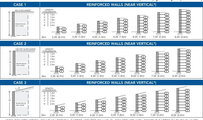
\*FOR CONSTRUCTION OF NEAR VERTICAL BATTER (CENTER PIN HOLE), CONSTRUCT WITH POSITIVE BATTER BY TILTING UNITS BACK TOWARDS FILL ON LEVELING PAD. ELEVATION DROP ALONG THE 10"(254mm) WIDTH OF THE BLOCK TO BE 3/8"(10mm).
